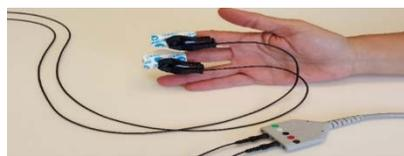
**Figure 8.** Attaching the EDA Transducer
